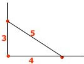
The goal is to bring the angle between the two marked sides to a perfect 90 degrees such that it measures exactly 5' when measured across the diagonal.
