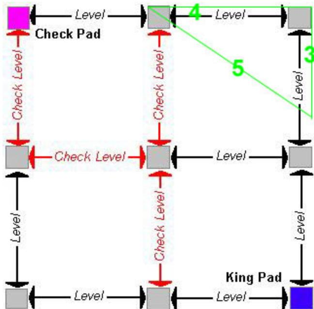
**8.** From here level each successive pad around the perimeter. Go both directions around the perimeter until you get to the pad diagonally across from the king pad. Level this last block from one side and check its level from the other side.
